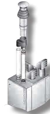
Balanced flue roof outlet (type C32)
